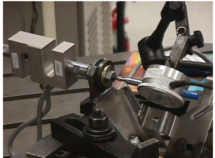
Figure 1. To test the bending stiffness of a shift cable holding bracket, the S-shaped load transducer (left) measures applied load while the dial indicator (right) measures displacement as the bracket flexes. Both devices are candidates for TEDS. Photo courtesy of NSK Steering Systems America Inc.
