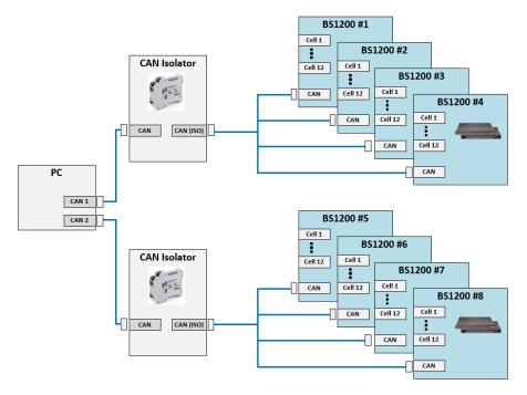
Figure 4: Install one CAN isolator per 2-4 Battery Simulator 1200s when CAN communications are used.
