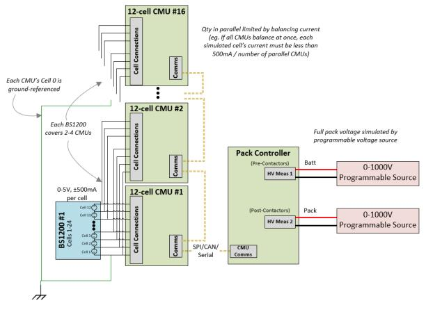
Figure 7: Low-voltage, shared cell simulation: simulated cell channels are shared among multiple CMUs, each CMU is ground-referenced, and high voltages are simulated by programmable sources.
