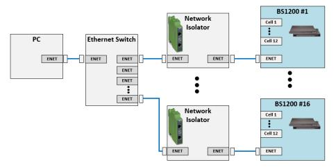
Figure 3: Install one network isolator per Battery Simulator 1200 when the Ethernet port is used or connected.
