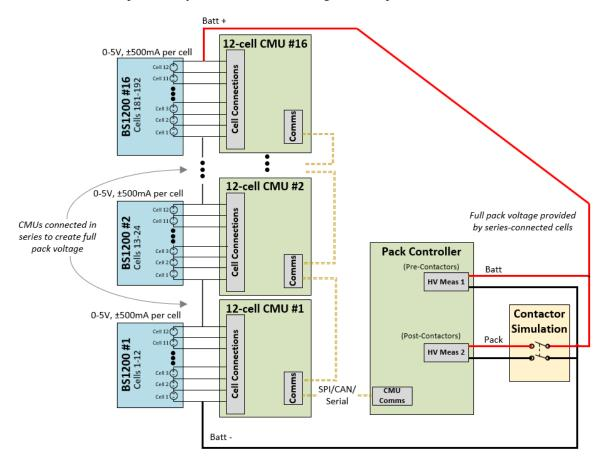
Figure 5: Full stack simulation: all cells are individually simulated, controlled and connected in series, most similar to an actual battery stack.
