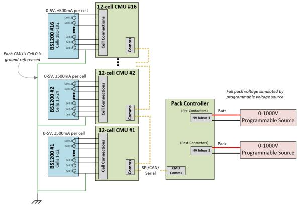
Figure 6: Low voltage, full cell simulation: all cells are individually simulated and controlled, though each CMU is groundreferenced. High voltage is simulated by external programmable sources.
