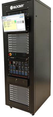
Note that the Battery Simulator 1200 will withstand abrupt power loss without damage, though any networked computer or controller will lose communication and may require an application reset, restart or reboot depending upon how the software is written to handle communication loss. Typically, CAN communications will restart automatically once the Battery Simulator 1200 powers up.
