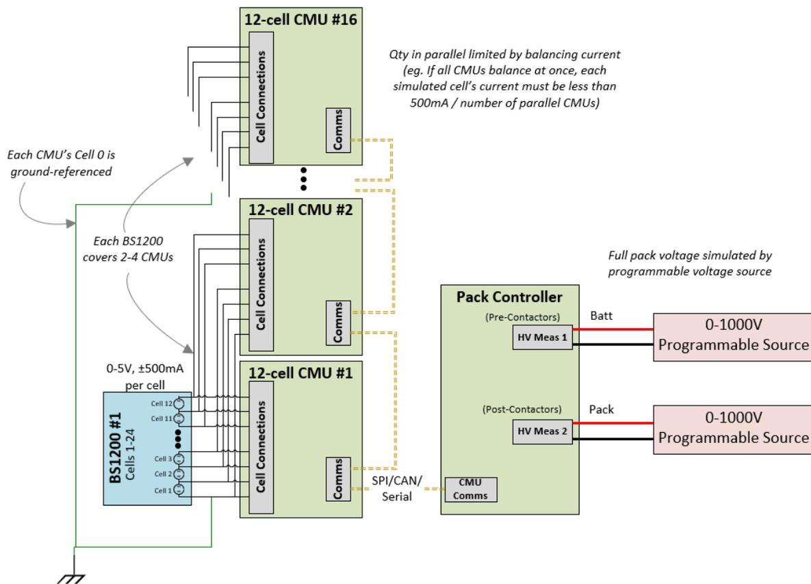
Figure 7: Low-voltage, shared cell simulation: simulated cell channels are shared among multiple CMUs, each CMU is ground-referenced, and high voltages are simulated by programmable sources.
