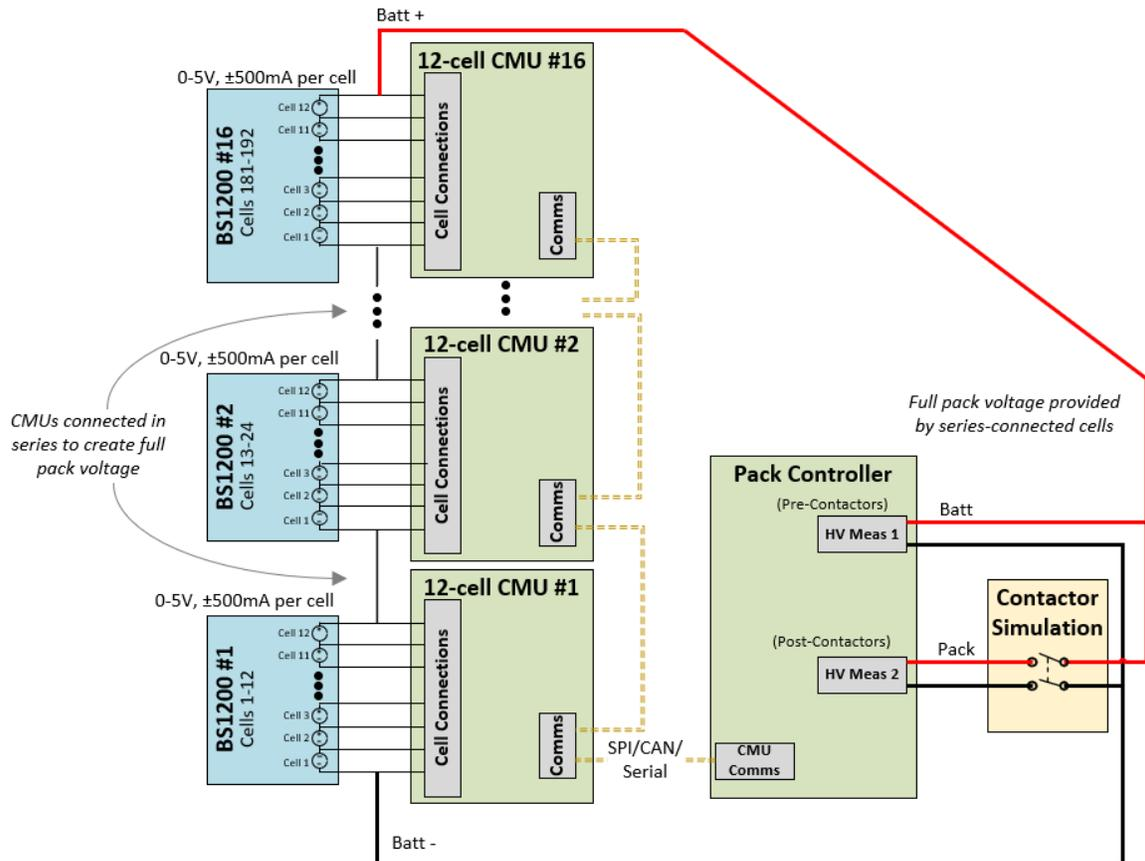
Figure 5: Full stack simulation: all cells are individually simulated, controlled and connected in series, most similar to an actual battery stack.
