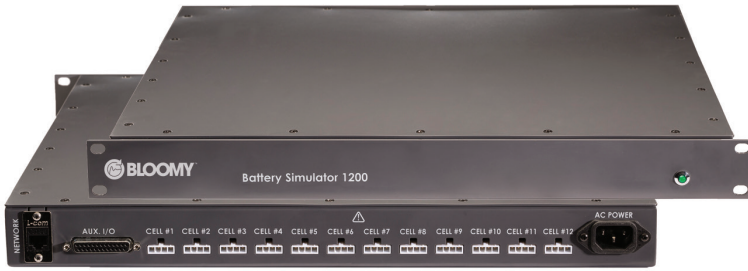
Bloomy's Battery Simulator 1200 product. 12 simulated cells packaged in a rack-mountable enclosure for mounting in standard equipment racks. The cell terminals are 4-wire cable assemblies to sense and feedback the cell voltage where they connect to the BMS.
