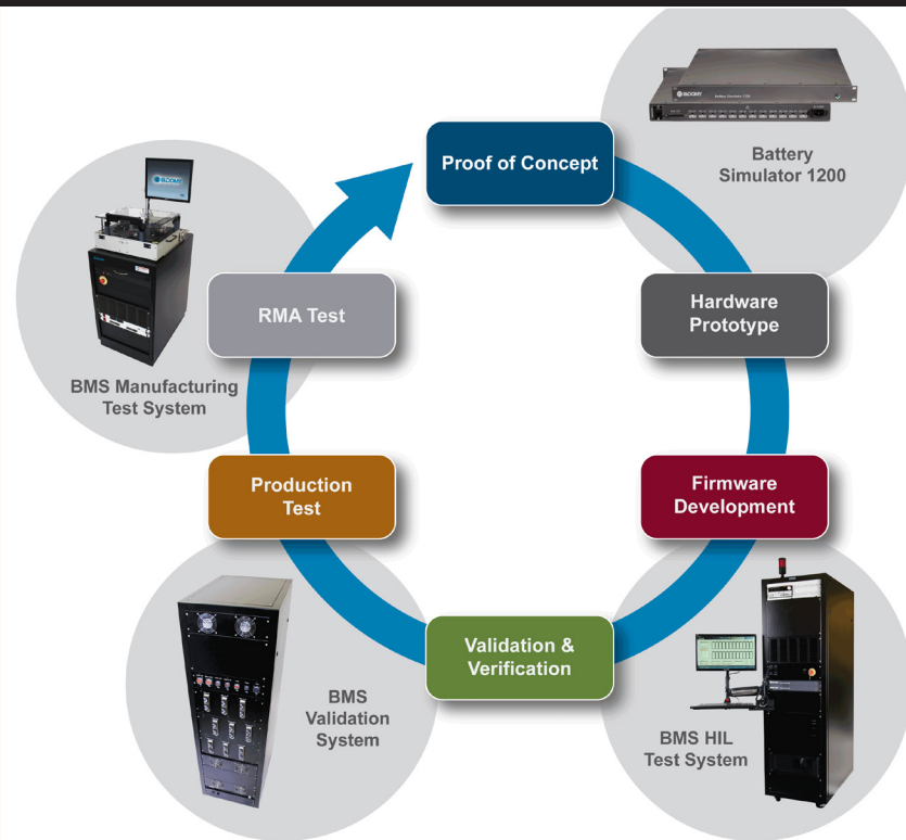
The BMS development lifecycle and the types of testing equipment that is performed at each stage.
