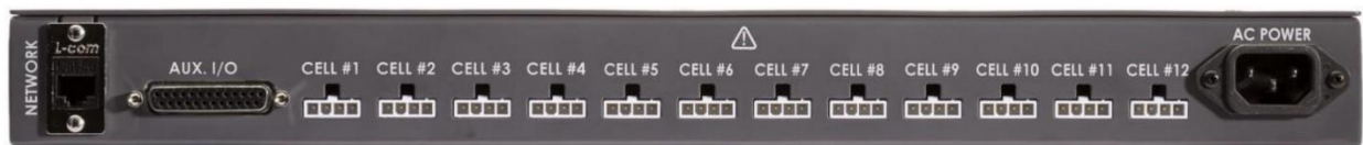
Figure A.2: The rear panel of the Battery Simulator 1200/1201 contains the network connector, cell connectors and the Auxiliary I/O connector. Prevent access to these connectors when high voltages are present.
