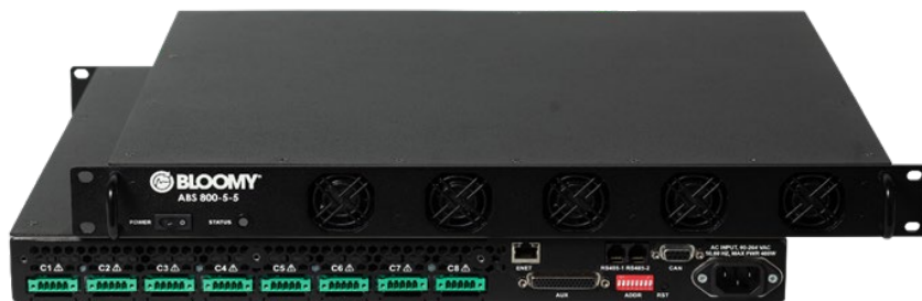
Figure 3. The Advanced Battery Simulator 800 is an 8-Cell battery simulator in a 1U rackmount enclosure that can also run a cell model and perform short, open and reverse-polarity faults onboard.
